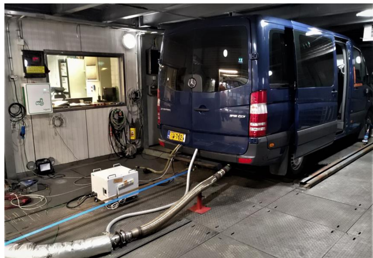
Emissions and fuel consumption test facility with a single-roller 2WD dynamometer and Mercedes van retrofitted with Proventia NOxBUSTER
