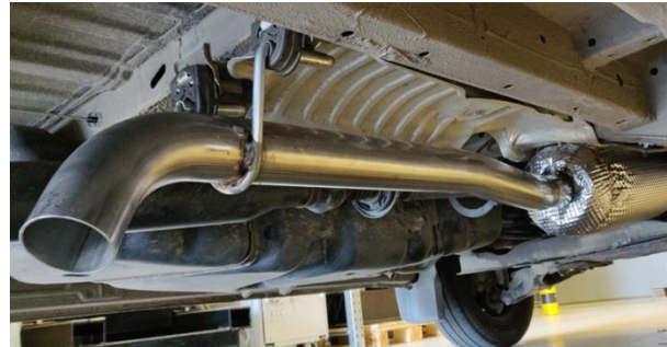
Test: NOxBUSTER City Light retrofit SCR system installed to vehicle
