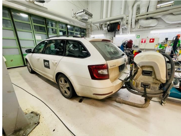
Figure 25: Skoda Octavia Diesel (test vehicle #2) with the PEMS device installed
