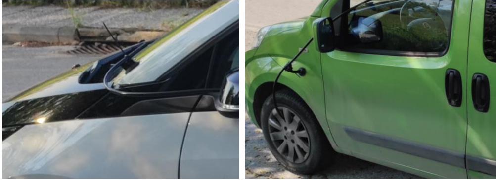
Figure 30: Inlet probe location during background measurements (left) and inlet probe placement for the brake particle counting (right)
