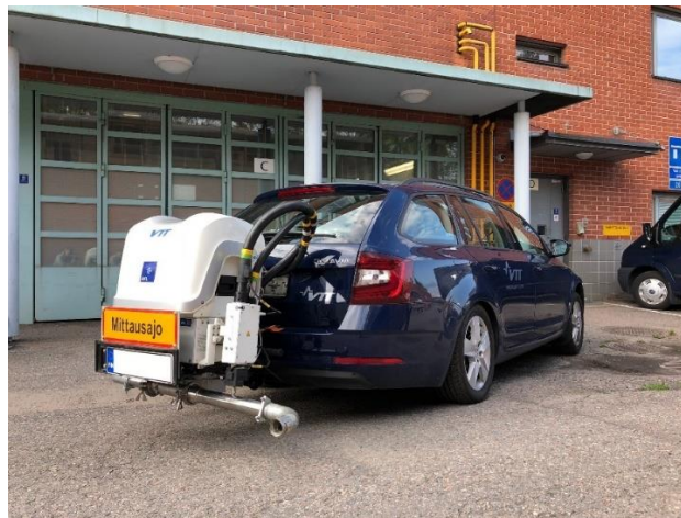
Figure 24: Skoda Octavia Petrol (test vehicle #1) with the PEMS device installed
