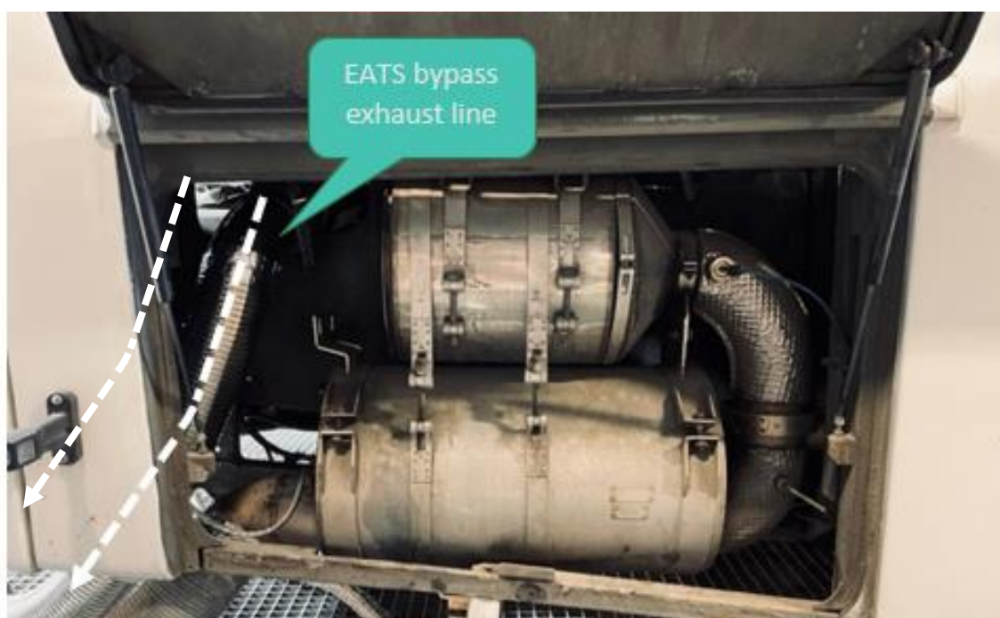
Figure 23: Tampered EATS bypass route to CVS tunnel (with normal route depicted in figure 2-3 now disconnected)
