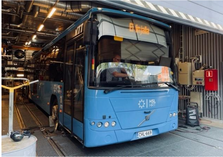
Figure 20: Test vehicle installed in the HD-chassis dynamometer environment
