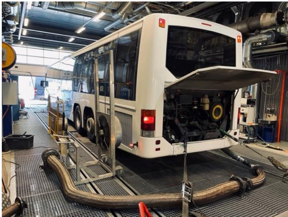
Figure 21: Test vehicle placed in the test cell
