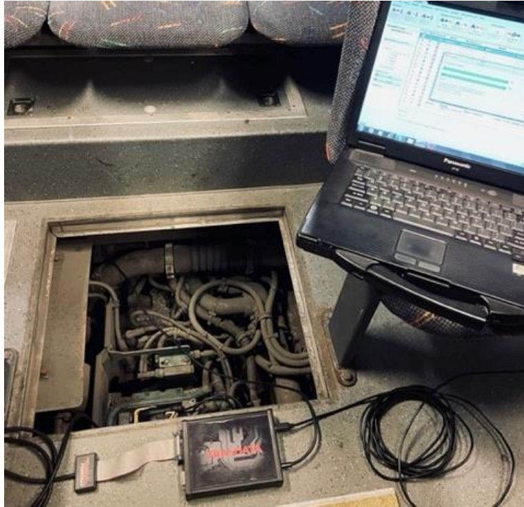
Figure 19: Illustration of the ECU reprogramming process
