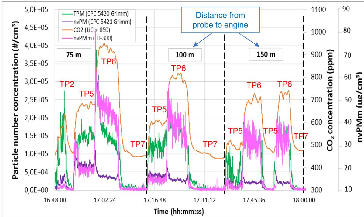
Power Engine from Flight Idle up to 80% N1
