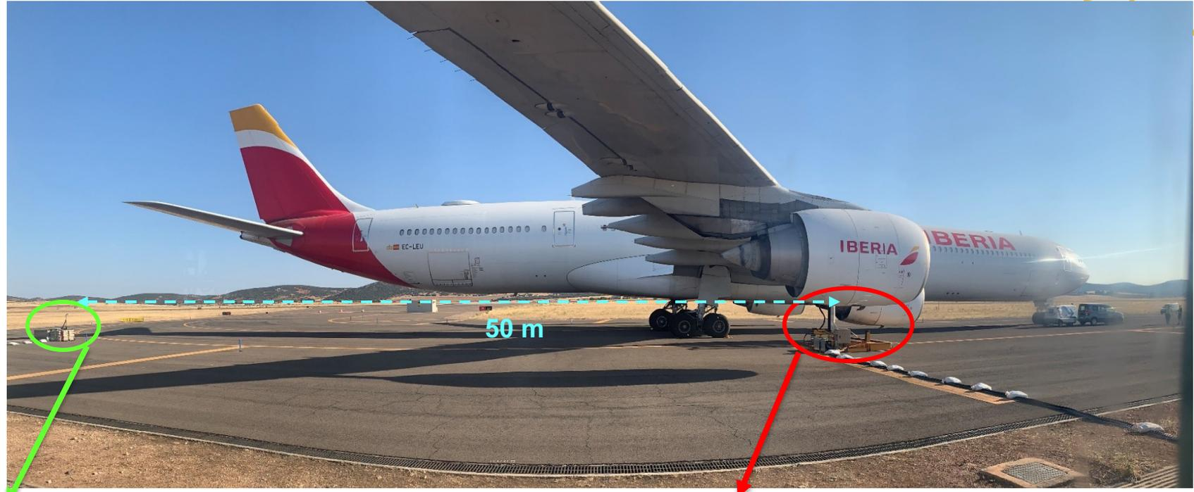
To measure on-wing main engine emissions at engine exit and downstream plume.
