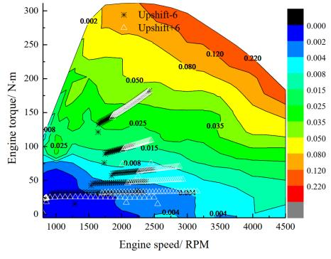
Figure 3.13: Engine operation points in NOx emission map
