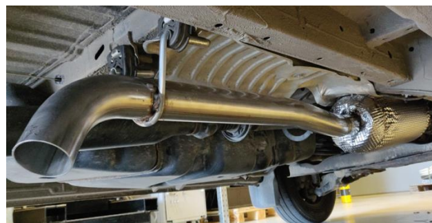
Figure 0.2: NOxBUSTER City Light retrofit SCR system installed to vehicle
