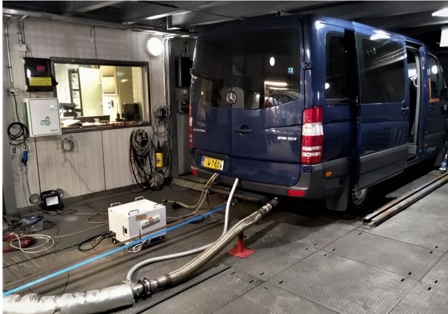
Figure 0.3: Emissions and fuel consumption test facility with a single-roller 2WD dynamometer
